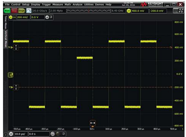
10. Runt-trigger mode quickly identifies and displays the runt event in the signal.
