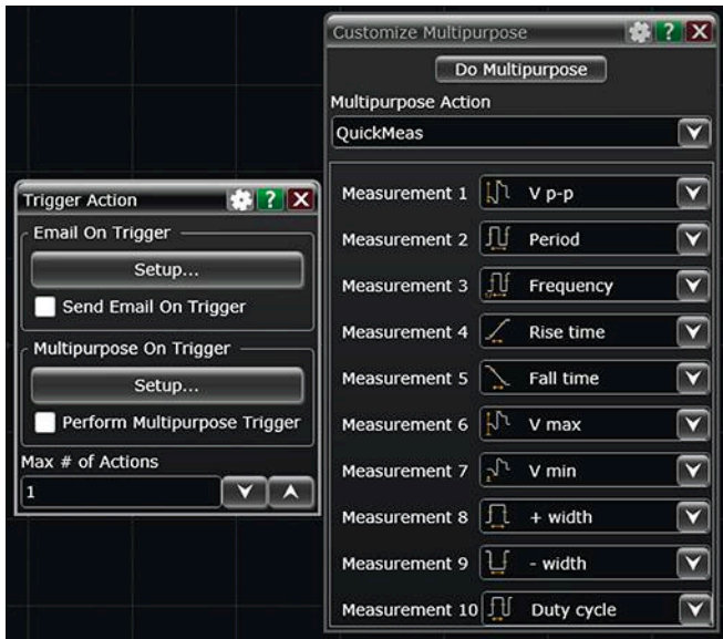
12. A wide variety of trigger actions are available on a Keysight Infiniium S-Series oscilloscope.
