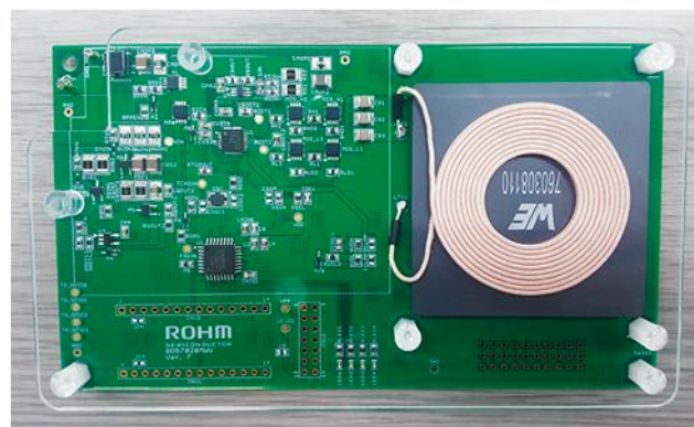
The BD57020MWV works as a controller in the wireless power transmitter based on the Qi compliant by using it with a general-purpose microcomputer. (Courtesy of Wireless Power Consortium)
