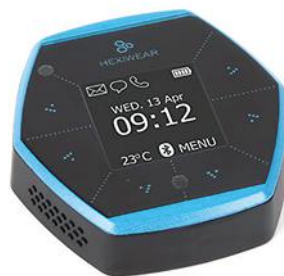
2. The Hexiwear module (left) runs a NXP Kinetis K64x Cortex-M4. It can be customized using a built-in header (right).
