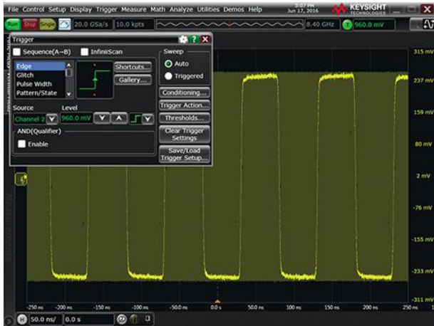
3. An inappropriate trigger configuration will cause triggers to occur on a predetermined time interval, regardless of signal behavior if auto-trigger is enabled, as seen here. Infinite-persistence has been enabled on Channel 1 to better illustrate what is occurring.
