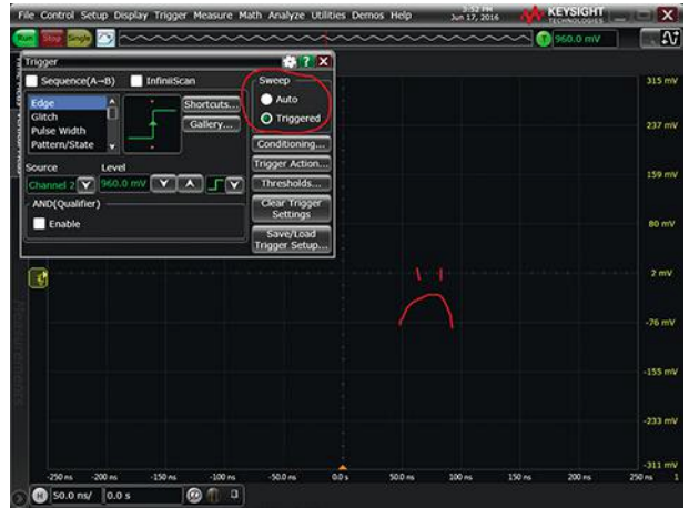
4. Disabling the auto-trigger feature without an appropriate trigger configuration means the oscilloscope won’t acquire at all.
