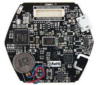
2. The Hexiwear module (left) runs a NXP Kinetis K64x Cortex-M4. It can be customized using a built-in header (right).
