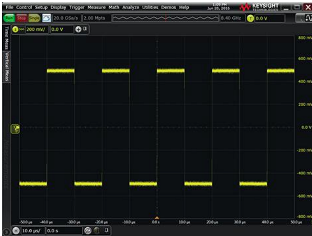
7. Edge-trigger mode isn't a good tool to use when searching for runt events in your signal.
