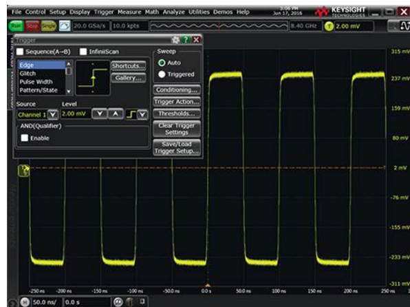
2. Auto Scale automatically configures the oscilloscope to trigger on the rising edge of Channel 1.
