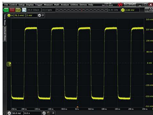
1. Using Auto Scale on the oscilloscope produces this view of a 10-MHz square wave.
