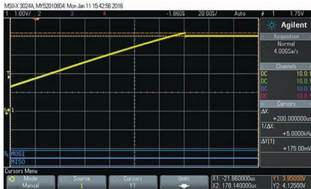
3. The clamping action is small but effective, as shown by this “zoom in” view of the output.
